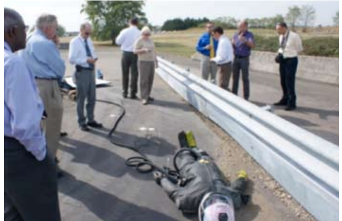
Figure 12 Members of the FHWA/AASHTO Motorcycle Scan Team witnessed the crash test of a “dummy” into a motorcycle guardrail at 60 km/h at the French National Institute for Transport and Safety Research in September 2010. Photo – J. Baron
